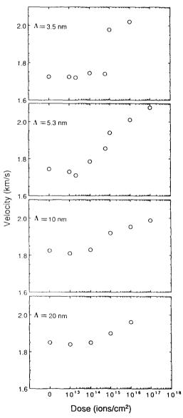
Fig. 2. Acoustic phonon velocities of the superlattice samples as a function of irradiation dose with 6 MeV Si<sup>+</sup> ions.
