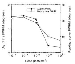
Fig. 6. Ag(111) peak and rocking curve FWHM values vs. irradiation dose for the 20.0 nm modulation wavelength sample.
