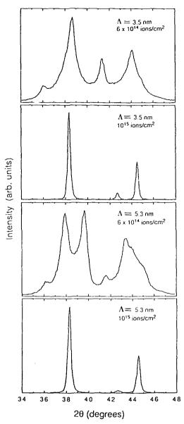
Fig. 5. X-ray diffraction spectra, at ion doses of  $6 \times 10^{14}$  and  $10^{15}$  ions cm<sup>-2</sup>, for the 3.5 and 5.3 nm modulation wavelength samples.
