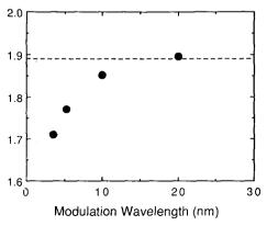
Fig. 1. Acoustic phonon velocities of the unirradiated superlattices as a function of modulation wavelength.
