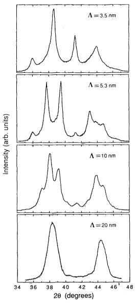
Fig. 4. X-ray diffraction spectra, prior to irradiation, for the modulation wavelengths used in this study.
