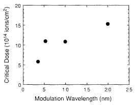
Fig. 3. Plot of the irradiation dose required to attain the inflection point in the phonon velocity *vs.* irradiation dose plot ("critical dose") *vs.* modulation wavelength.
